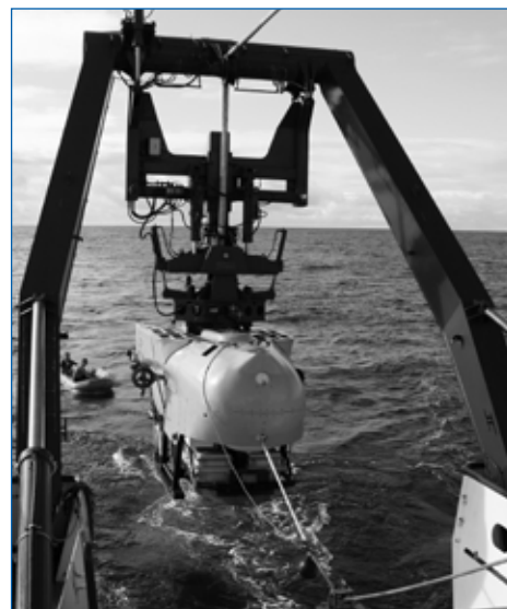
The PISCES V research submersible being launched from the R/V Ka'imikai-o-Kanaloa during a research expedition Tom Guilderson participated in near Hawaii
